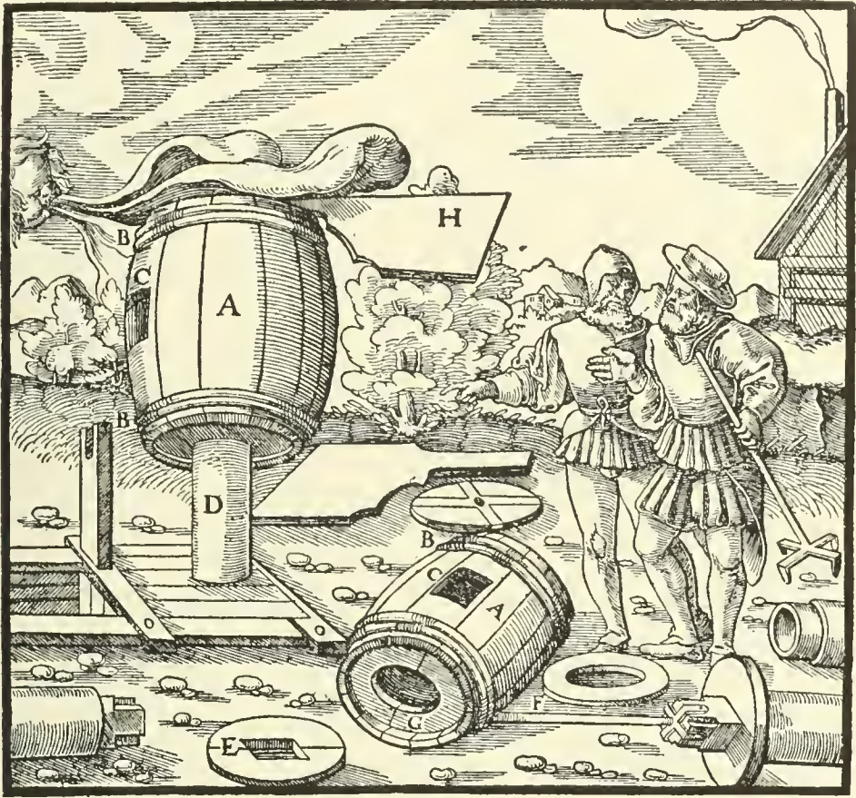
A—WOODEN BARRELS. B—HOOPS. C—BLOW-HOLES. D—PIPE. E—TABLE. F—AXLE. G—OPENING IN THE BOTTOM OF THE BARREL. H—WING.
